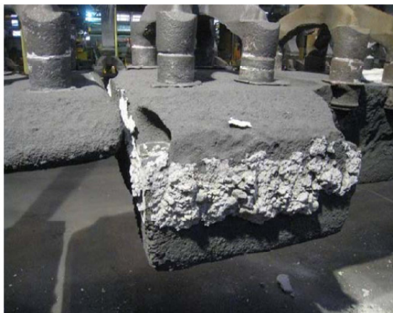
Figure 2. Spent anode, stub, thimble & bath.
