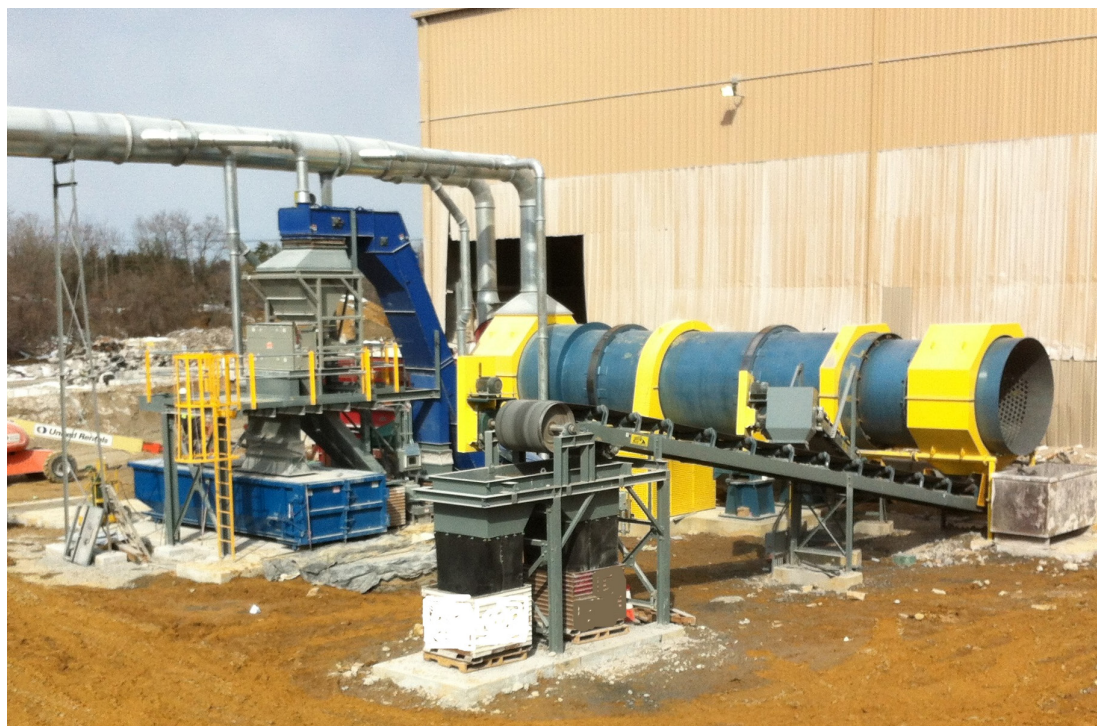
Figure 1. DIDION RT 108 DIDION Crusher / Metal Separator.
